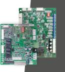
Base Control (ABC) offers two way communication between components, advanced operating logic and robust troubleshooting capabilities. The Aurora Expansion Board (AXB) adds support for true energy monitoring and Symphony compatibility. AXB also expands communication to include the internet, the smart grid, home automation networks and our IntelliZone2 zoning system.
